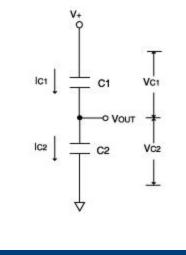
If IC1 > IC2 VOUT rises until IC1 = IC2 If VC2 = VOUT > 2.7V, C2 is damaged due to over – voltage Total leakage current equals IC1.
