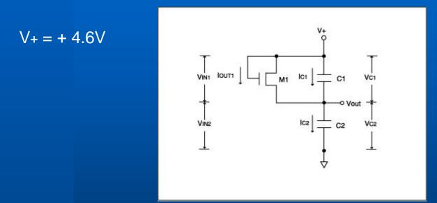
If IC2 > IC1 VOUT drops until M1 is turned on M2 is turned off, IOUT2 is zero IOUT1 + IC1 = IC2 VOUT  $\sim$ = 2.25V for IC2  $\sim$ = 10 x IC1 Total leakage current equals IC2 at 2.25V.
