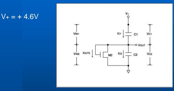
If IC1 > IC2 VOUT rises until M2 is turned on M1 is turned off, IOUT1 is zero IOUT2 + IC2 = IC1 VOUT  $\sim$ = 2.35V for IC1  $\sim$ = 10 x IC2 Total leakage current equals IC1 at 2.25V.
