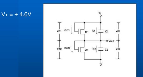
When IC1 = IC2 VOUT ~= 2.30VM2 is slightly turned on M1 is slightly turned on IOUT1 + IC1 = IOUT2 + IC2 Pick minimum IOUT1 value so that IOUT1 << IC1 Total leakage current equals ~ IC1
