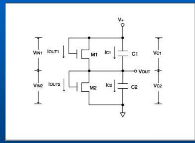
M1 connects across C1, VIN1 = VC1 M2 connects across C2, VIN2 = VC2 V+ = VIN1 + VIN2 = VC1 + VC2 IC1 + IOUT1 = IC2 + IOUT2
