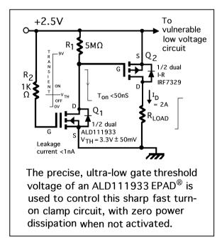
The actual clamp voltage is adjustable within a certain range by varying the value of  $R_1$  (i.e. 500K $\Omega$  to 20M $\Omega$ ), which allows a limited adjustment of precisely when the circuit turns on. This ability to turn on at slightly higher/lower gate-to-source voltages is due to the EPAD's unique precision, and enables the user to set the turn-on clamp voltage at a very precise level, which could be very close to the normal operating point of the circuit.
