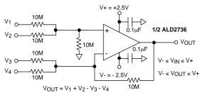
$R_{IN}$  = 10M $\Omega$  Accuracy limited by resistor tolerances and input offset voltage
